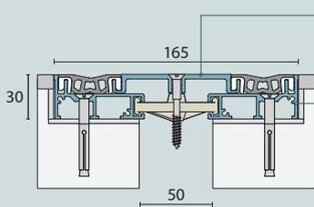
Flush aluminium centre plate is natural anodised as standard.
