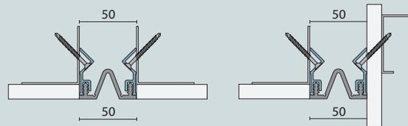
The frame configuration of FWS-M options suits both wall to wall and corner wall situations.
