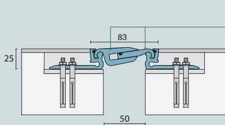
Interlocking cover design allows for multi-directional movement.
