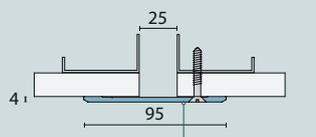
Smooth cover plate is supplied in a natural anodised finish, or can be polyester powder coated<sup>^</sup> to match the surrounding finishes.
