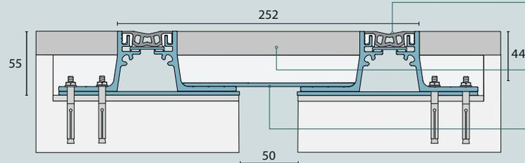
Smooth TPR gaskets are suitable for areas where hygienic finish is required. They are installed with a continuous aluminium support plate underneath for added durability.
