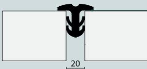
KP seals are bonded to the substrate using a neoprene adhesive (by others).
