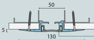
Single gasket expands and contracts during movement and is held in position by the aluminium side frames.
