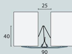
W-90 installed over 25mm joint width using small clip option.
