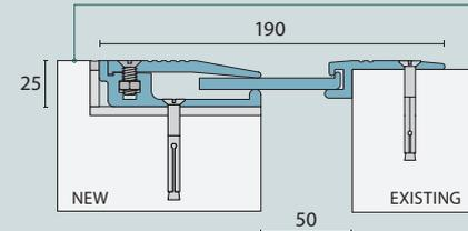
FFL at this point should be 6mm higher than the existing floor level.
