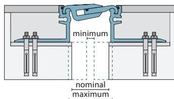
\* When material such as a fire barrier, or joint cover parts are situated within the joint opening, it is important to avoid using '0' [zero] as the minimum joint width. Any such part would get damaged if a joint closed to 0mm.
