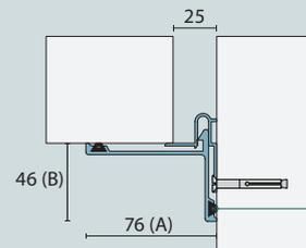
Gaskets on cover edges allow for optimal fit to the wall.
