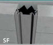
SF  | Flush gasket design; large range of sizes; multi-directional movement      | SF ▶ 82    | up to 150mm**        | up to +75/-90mm            | All exteriors / All finishes | Fire Barriers ▶ 90-91<br>Moisture Barriers<br>▶ Supplied as standard<br>Acoustic Barriers ▶ 93 |
