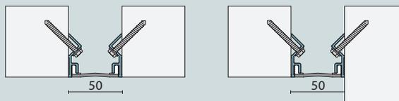
The frame configuration of FWF-M options suits both wall to wall and corner wall situations.
