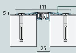
Aluminium side frames are designed to provide a minimal bump.
