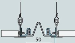
Aluminium frames attach directly to the ceiling grid for ease of installation.
