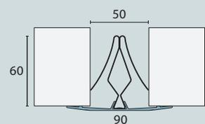
W-90 installed over 50mm joint width using large clip option.
