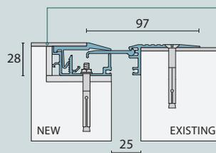
FFL on this side should be 5mm higher than the existing floor level.
