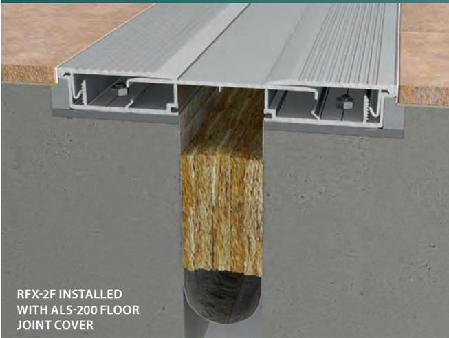
RFX-2F INSTALLED WITH ALS-200 FLOOR JOINT COVER
