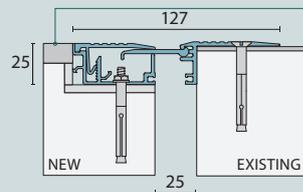
FFL on this side should be 2mm higher than the existing floor level.
