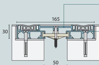
Recessed centre plate takes up to 3.2mm thick floor finish for maximum concealment.
