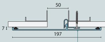
Cover plate is supplied in a natural anodised finish, or can be painted or supplied powder coated\* to match the surrounding wall finish.
