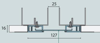
Free-floating aluminium centre plate spans joint opening and slides between side frame assemblies to allow movement when required.
