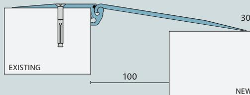
Vertical movement can only be accommodated on one side of the opening and only in one direction. Maximum allowable offset is 30mm.
