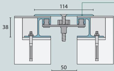
Stainless steel cover plates have a dull polished finish. The plates are self-centring to allow for movement when required.
