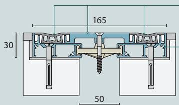
Extra thick centre plate and heavy duty gaskets will tolerate heavy rolling loads.
