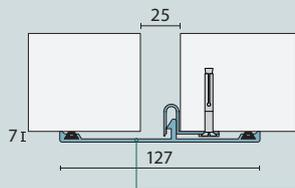
Cover plate snaps into a continuous anchor clip for simple installation.
