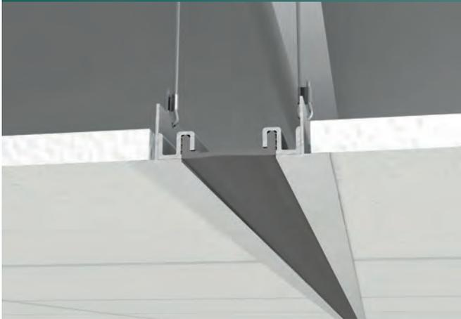
Suspended ceiling joint covers featuring flush gaskets for minimal visual impact.
