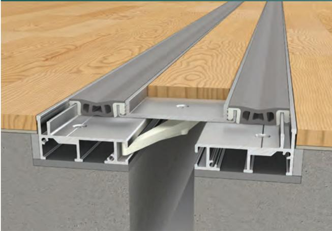
Recess mounted, concealed flush floor covers, with a centre plate designed to take floor finishes of up to 9.5mm thick<sup>^</sup>.
