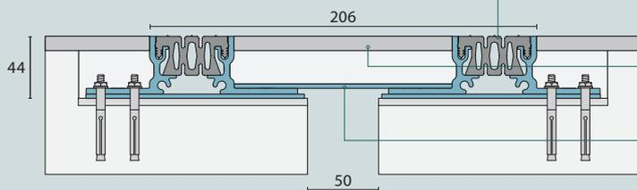
Heavy duty PVC gasket is suitable for areas with intensive pedestrian and wheeled traffic.
