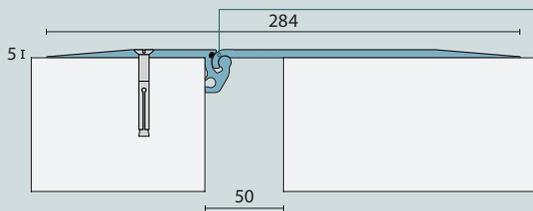
Cover is fixed to one slab, allowing movement over adjacent slab. Interlocking cover design allows for an offset in floor elevation.
