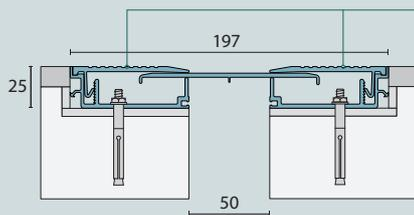
Serrations on cover plates create a slip resistant surface finish.
