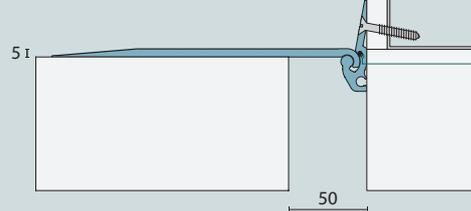
Water resistant rubber gasket eliminates any metal-to-metal noise.
