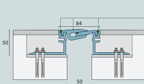
Exposed sections are serrated for a slip resistant finish.
