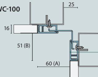
Cover plates clip into base frames to create a flush, tamper-resistant finish with no exposed fasteners.
