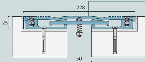
Secondary centre plate for increased durability and smoother transition in areas where trolley traffic is prevalent.
