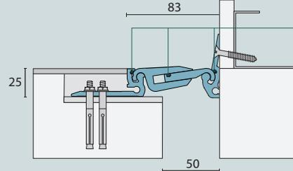
Water resistant rubber gaskets eliminate any metal-to-metal noise.
