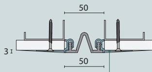
Aluminium frames are recessed to allow for taping and jointing, minimising visible joint surface.
