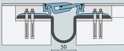
Acoustic Barrier is positioned in the joint opening, underneath the selected joint cover.
