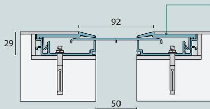
Recessed cover plates take up to 3mm thick vinyl finish for reduced visual impact.
