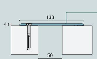
Single plate design is anchored to one slab, allowing movement over the adjacent slab.
