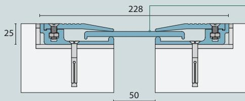
Free-floating centre plate spans joint and slides between frame assemblies to allow movement when required.
