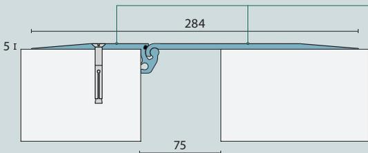
Serrated profiles provide slip resistant surface.
