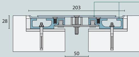
Dull polished stainless steel cover plate and bearing plates.
