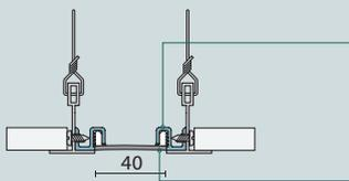
Aluminium frames attach directly to the ceiling grid for ease of installation.
