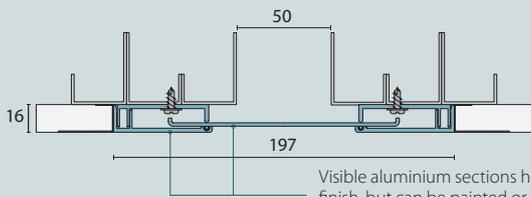
Visible aluminium sections have a natural anodised finish, but can be painted or supplied powder coated\* to match the surrounding wall finishes.
