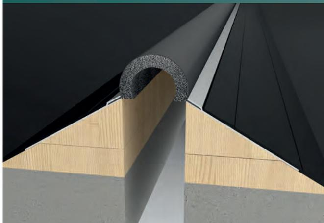
Flexible, weatherproof roof joint covers offering multi-directional movement.
