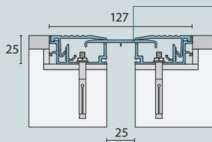
Free-floating centre plate spans joint opening and slides between frame assemblies to allow movement when required.
