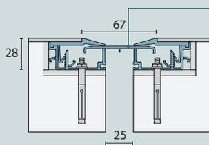
Free-floating centre plate spans joint opening and slides between frame assemblies to allow movement when required.
