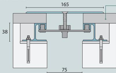
SJP series models can accommodate up to 25mm thick floor finish.
