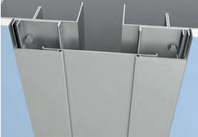
Durable metal joint covers for interior applications where low maintenance or tamper resistance are required.
