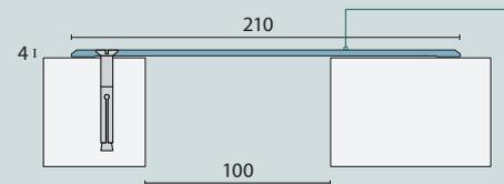
As standard, the aluminium plate is supplied in a natural anodised finish. Stainless steel version is available.
